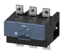
Overload relay 55...250 A for motor protection Size S10/S12, CLASS 5...30E Contactor mounting/stand-alone installation Main circuit: busbar connection Auxiliary circuit: Spring-type terminal Manual-Automatic-Reset Internal ground fault detection
