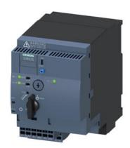
SIRIUS Compact load feeder Reversing starter 400 V 24 V AC/DC 50...60 Hz 8...32 A IP20 Connection main circuit: plug-in, without terminals Connection control circuit: Spring-type terminal
