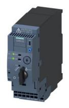
SIRIUS Compact load feeder DOL starter 690 V 24 V AC/DC 50...60 Hz 8...32 A IP20 Connection main circuit: plug-in, without terminals Connection auxiliary circuit: Spring-type terminal
