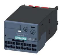
solid-state time-delayed auxiliary switch, ON-delay, relay: 1 CO, time range 0.05-100 s, 24-240 V AC/DC, 50/60 Hz, varistor for attenuation of the contactor coils integrated, spring-loaded terminal, can be snapped on at the front on contactors 3RT2 and auxiliary contactors 3RH2
