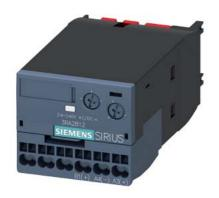
electronic timing relay, off delayed, with control signal and semiconductor output, time range 0.05-100 s, 24-240 V AC/DC, 50/60 Hz, varistor for attenuation of the contactor coils integrated, spring-loaded terminal, can be snapped on at the front on contactors 3RT2.1 / 3RT2.2 and auxiliary contactors 3RH2
