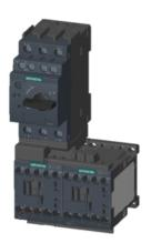
Fuseless motor starter Reversing operation 600VAC Size S00 1.1-1.6A 24V DC screw connection For screw mounting Or 35 mm rail-mounting Type of coordination 2 IQ = 150 KA Also full fills type Of coordination 1 1NO+1NC (MSP) 1NC (per contactor)
