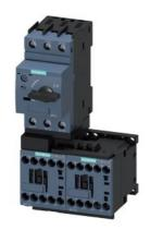
FUSELESS LOAD FEEDER REVERSING OPERATION, AC 400V, S00 1.1...1.6A, AC 110/120V 50/60HZ SCREW TERMINAL FOR RAIL MOUNTING, TYPE OF ASSIGNMENT 2,IQ = 150KA (ALSO FULFILLS TYPE OF ASSIGNMENT 1) 1NC (CONTACTOR)
