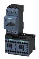
Fuseless motor starter Reversing operation 600VAC Size S00 0.11-0.16a 110/120VAC 50/60HZ screw connection For screw mounting Or 35 mm rail-mounting Type of coordination 2 IQ = 150 KA Also full fills type Of coordination 1 NC (per contactor)
