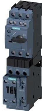
Fuseless motor starter Direct start 600VAC Size S0 5.5-8Amp 110/120VAC 50/60HZ screw connection For screw mounting Or 35 mm rail-mounting Type of coordination 2 IQ = 150 KA Also full fills type Of coordination 1 1NO+1NC (MSP) 1NO+1NC (contactor)
