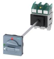
SENTRON, Molded case switch 3LD5 UL, Main switch, 3-pole, certified according to UL489 UL60947-4-1 and IEC60947-3, UL: 60A, SCCR 50kA at 480VAC, Operating power at 480VAC 3-phase: 40hp, IEC: 63A, Operating power at AC-23A at 400V: 30kW, floor mounting with door coupling rotary operating mechanism, defeatable, Standard, 4-hole mounting of the handle, without tolerance compensation, incl. terminal covers for the infeed side
