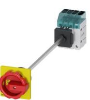
Load disconnector 3LD3, lu 32 A Main switch 3-pole + N Rated operating capacity for AC-23 A at 400V 11.5kW floor mounting Basic switch with door coupling Central hole mounting 22.5mm Rotary actuator red / yellow 66 x 66 mm
