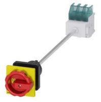
SENTRON, Switch disconnector 3LD, emergency switching-off switch, 3- pole, lu: 32 A, operating power / at AC-23 A 400 V: 11.5 kW, floor mounting with door coupling, rotary operating mechanism, Red / yellow, central mounting 22.5 mm of the handle
