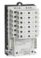
Electrically held lighting contactor, (convertible to mech. held), Amp rating 30A (tungsten 20A), 1 N.C. / 1 N.O. poles, 460-480V 60Hz/440V 50Hz coil, Non-combination type, Enclosure NEMA type (open), No enclosure
