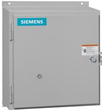
Non-reversing contactor, Size 1 3/4, 4 power poles, Contactor amp rating 40A, 3 wire (NO aux included), 110V 50Hz / 120V 60Hz coil, Non-combination type, Encl. NEMA type 4X fiberglass, Water/dust tight noncorrosive, Standard width enclosure
