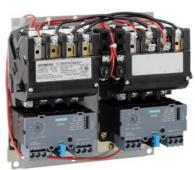
2-speed 3-phase motor starter Size 3 Two separate windings Constant or variable torque Solid-state overload relays Low SPD OLR range 13-52a High SPD OLR range 25-100A 110-120/220-240VAC 60HZ coil Enclosure NEMA type (open) No enclosure
