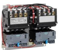
2-speed 3-phase motor starter Size 1 Two separate windings Constant or variable torque Solid-state overload relays Low SPD OLR range 5.5-22A High SPD OLR range 10-40a 110-120/220-240VAC 60HZ coil Enclosure NEMA type (open) No enclosure
