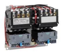
2-speed 3-phase motor starter Size 0 Two separate windings Constant or variable torque Solid-state overload relays Low SPD OLR range 0.75-3.4A High SPD OLR range 0.75-3.4A 110-120/220-240VAC 60HZ coil Enclosure NEMA type (open) No enclosure
