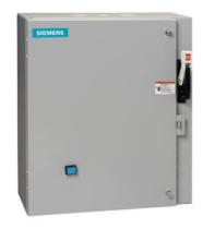
Non-reversing motor starter, Size 2, Three phase full voltage, Solid-state overload relay, OLR amp range 13-52A, Combination type, 50A circuit breaker, Enclosure NEMA type 1, Indoor general purpose use, Extra-wide enclosure
