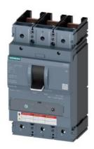
circuit breaker 3VA5 UL frame 400 breaking capacity class C 100kA @ 480 V 3-pole, line protection TM240, ATAM, In=250A overload protection Ir=175A ...250A short circuit protection Ii=5...10 x In w/o connection
