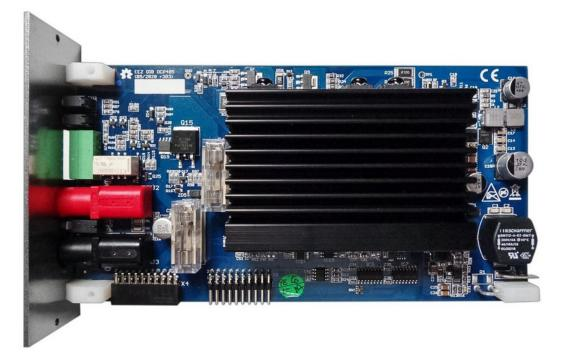
The DCP405 power module is programmable DC source for EEZ BB3 T&M chassis that can deliver up to 40 V and 5 A (max. 155 W) using the hybrid topology of switching pre-regulator and linear (series) post-regulator for improved power efficiency and precise voltage and current setting and fast transient response.
