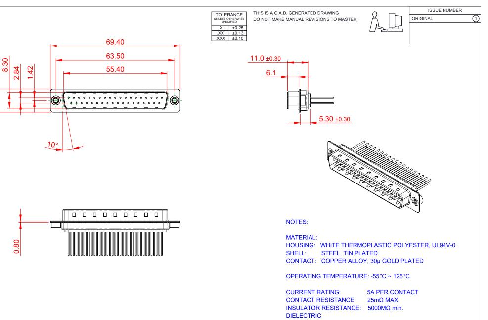
WITHSTANDING VOLTAGE: 1000V AC rms
