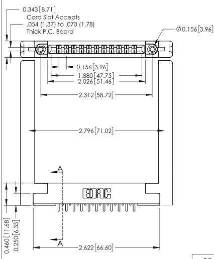
A-ASECTION 0.295 [7.49] Card Slot 0.165[4.19] Point of Contact
