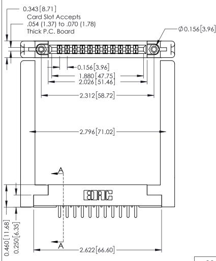
$\forall$ - $\forall$ SECTION 0.295 [7.49] Card Slot 0.165[4.19] Point of Contact
