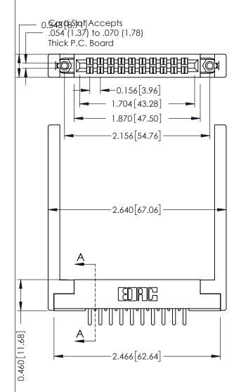
0.090[2.29] Point of Contact 305 ENG MASTER 305 / 315 / 355 Card Edge Connector J.LEE DATE: SEPT. 21/09 Part Number: 315-020-520-268 NTS SHEET 1 OF 2
