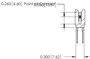
745 Series Ultra-Mate Card Edge Connector - Press Fit ACAD REFERENCE NO. Part Number: 745-106-540-206 **EDAC INC** THESE DRAWINGS AND SPECIFICATIONS
