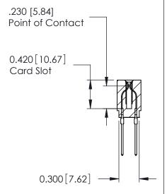
ACAD REFERENCE NO. 725-ENG MASTER 725 Series Ultra-Mate Card Edge Connector - Press Fit SEGAHON:3A:9A DRAWN: J.LEE Part Number: 725-030-545-201 CHECKED: DATE: **EDAC INC** SCALE: SHEET 1 OF 1 THESE DRAWINGS AND SPECIFICATIONS ARE THE PROPERTY OF EDAC INC.,AND TORONTO, ONTARIO SHALL NOT BE REPRODUCED, OR COPIED DRAWING NUMBER **ISSUE** CANADA OR USED AS THE BASIS FOR THE 725-ENG MASTER MANUFACTURE OR SALE OF APPARATUS YOUR CONNECTION TO QUALITY & SERVICE WITHOUT WRITTEN PERMISSION.
