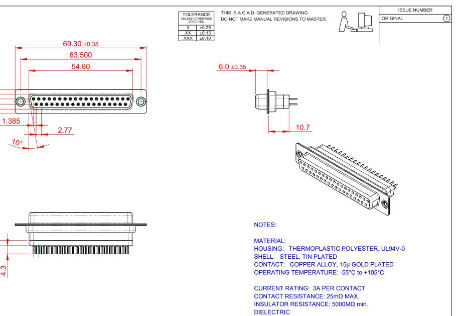
WITHSTANDING VOLTAGE: 1000V AC rms
