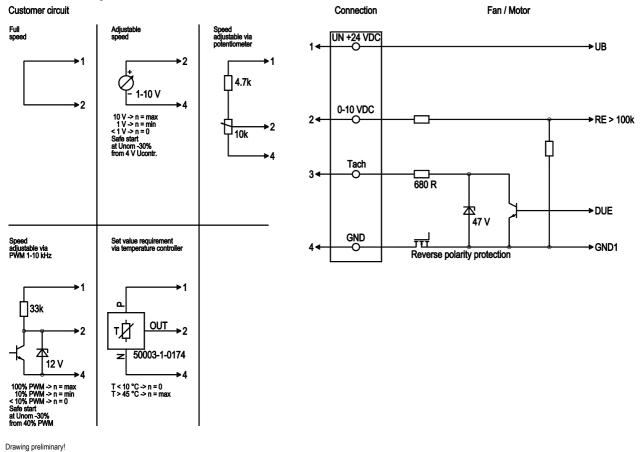
Conn. Designation Color No. Function/assignment Un +24 VDC Power supply 24 VDC, maximum ripple 3.5 % 1 1 red 2 0-10 VDC Control input Re > 100k 1 yellow Tach output, 3 pulses per revolution, Isink max = 10 mA 3 white 1 Tach GND 1 4 blue Reference ground
