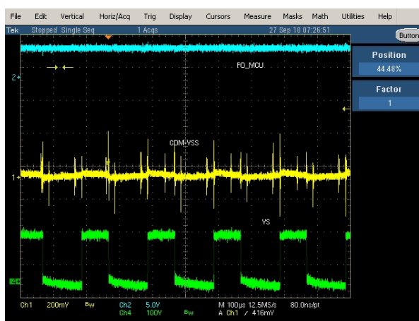
Figure 35. During startup current is high, with cap between COM-VSS, noise is less, fault conditions do not occur, compressor will not stall, 100us/div
