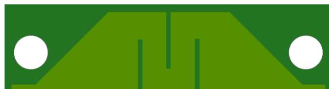
Figure 19. PCB Trace Design to Generate Differential Magnetic Field for CT453 to Measure
