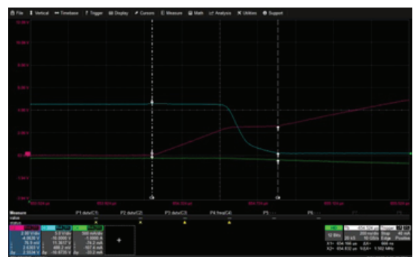
Figure 11: Turn-Off and Turn-On Behavior—C2 Power MOSFET, V_{GS} ; C3 Power MOSFET, V_{DS}
