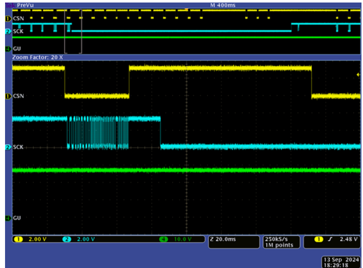
Figure 49: Short to GND Occurring When CSN is High (Zoomed-In View)
