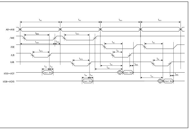
7. Write Cycle Timing 4 (/UB(/LB) Access)
