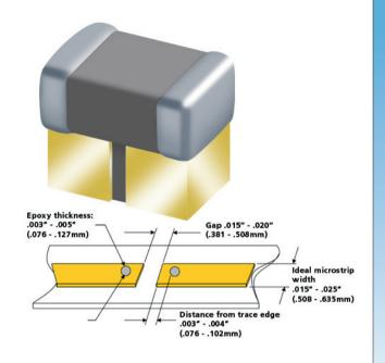
4. After the reflow step is completed, inspect joint for voids or excess flux and non-reflowed solder balls that can degrade performance or cause shorts across the gaps. Proper cleaning after the reflow process is crucial to avoiding performance degradation and discovering poor solder joints.
