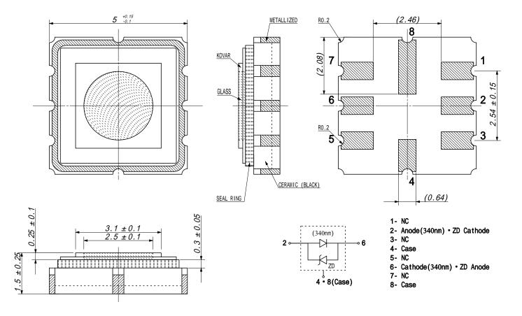
Recommended Soldering Pattern [mm]
