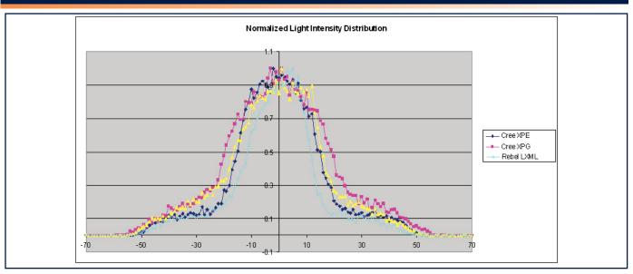
The full-width at half-maximum emission angle is:
