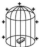
To complete the enclosure, make sure to place lids on boxes or containers, and close shielding bags. Packaging with holes, tears, or gaps should not be used as the contents may be able to extend outside the enclosure and lose their shielding as well as mechanical protection.
