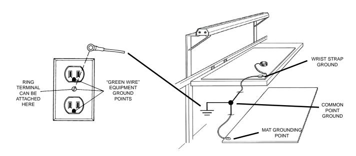
"The single most important concept in the field of static control is grounding. Attaching all electrically conductive and dissipative items in the workplace to ground allows built-up electrostatic charges to equalize with ground potential. A grounded conductor cannot hold a static charge." [Grounding ANSI/ESD S6.1Foreword]
