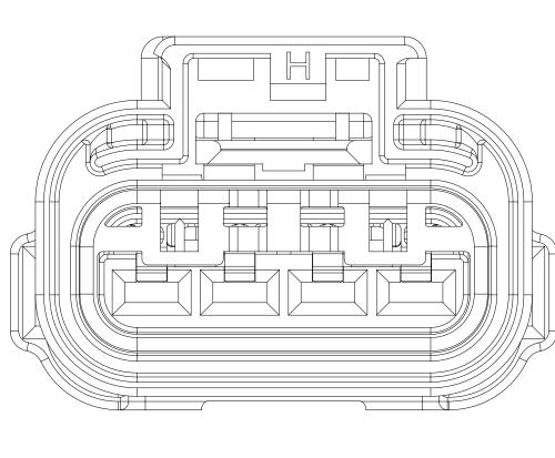
AUXILIAR FRONT VIEW type A - matt seal w/o holes
