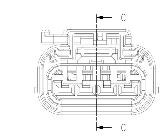
AUXILIAR FRONT VIEW TYPE B - SEALED (PARTIAL) ASSEMBLY SEE NOTE #5 - SHIPPED WITHOUT MATT SEAL AND RETAINER
