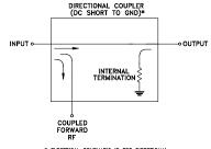
ELECTRICAL SCHEMATIC IS FOR DIRECTIONAL COUPLER WITH INTERNAL TRANSFORMER(S) THA POLITES DC FROM RF PORTS TO GROUND REV. A M151107 ED-8967A/1 DBTC-13-5-75X+ W7/CP/AM
