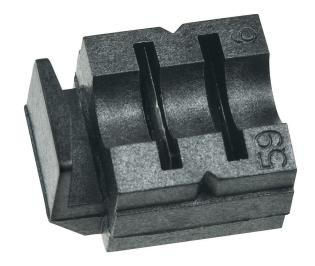
Designed for use with Klein's Radial Strippers. Two levels of blades strip RG59, RG6 and RG6 QS coaxial cable. Pre-set cutting blades for precise and accurate stripping. Durable high-carbon steel cutting blades are ground and honed for long life. Patented "V" notch eliminates scoring of the center conductor.
