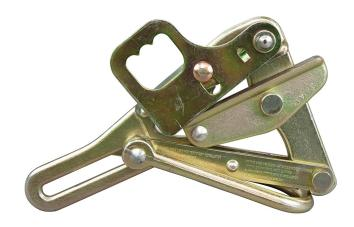
The Klein S1656-20H Chicago Grip-with Hot-Line Latch for Bare Conductors is for both bare and insulated conductors. The Klein S1656-20H Chicago Grip-with Hot-Line Latch for Bare Conductors may be placed on wire with hot-line stick. When stick is removed, latch closes automatically to guard against grip accidentally disengaging from wire.
