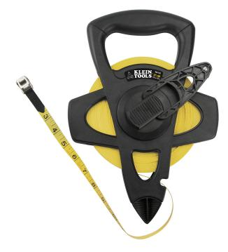
Klein Tools 150-Foot (45.72 m) Tape Measure is made from woven fiberglass tape with moisture-proof coating of polyvinyl chloride assures durability and protects against oil or chemicals. All metal parts are nickel plated for protection against rust. Tape line is graduated in feet and inches to 8ths.
