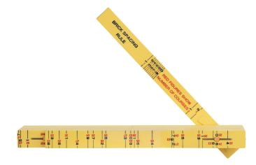
Klein Tools' 6-Foot Brick Fiberglass Folding Ruler is constructed of tough nylon, reinforced with glass fibers for added durability, and resistance to weather, abrasion, and most chemicals. Inch measurements are marked on both edges of the outside faces of the rulers, graduated to 1/16-Inch (1.6 mm). Standard brick scale measurements are marked on the inside faces of the rulers. Graduations are engraved on both sides with brick scale units on the other side for versatility.
