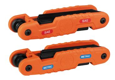
Klein Tools 2-Piece Pro Folding Hex Key Set features 21-Keys including SAE and metric Sizes. This set combines the 11 most common SAE sizes and 10 common metric sizes all in one set to tackle any job. The hex ends are square-cut for a secure full-depth fit and maximum contact with the hex socket to prevent slippage and stripping of the socket.
