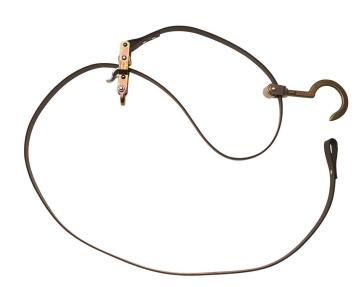
Sag service connections quickly with this simple proven tool. The strap is made of tough nylon webbing, and the swivel hook is forged steel. All metal parts are galvanized, and this tool has a 500-Pound (227 kg) maximum safe load.
