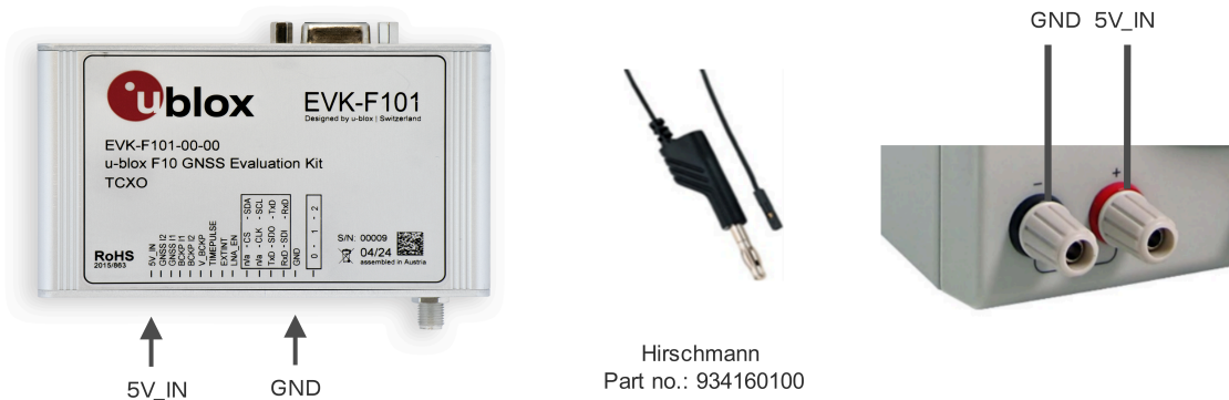
Figure 3: EVK-F101 5.0 V DC power supply example
