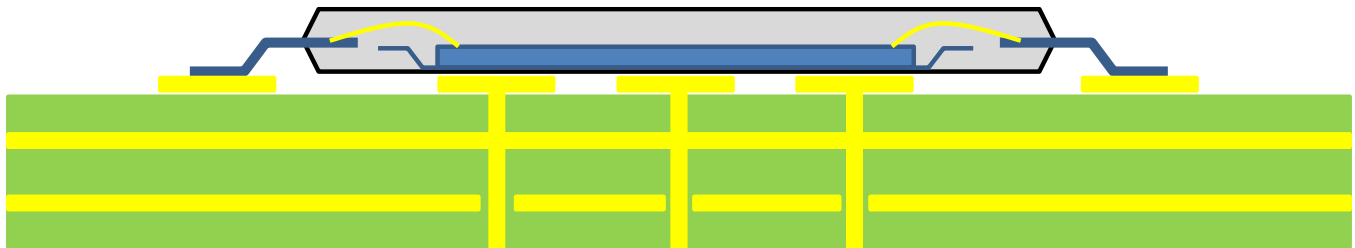
Figure10.2-1: Example thermal via holes on PCB.
