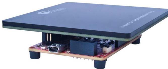
Figure 1-3: CY8CKIT-024 Connected to CY8CKIT-042
