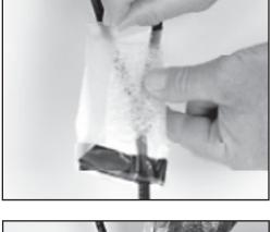
**4.7** Mix the resin per instructions on resin package. Pour into mold.
