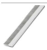
Band ferrules, 0.5 mm², sleeve length 8 mm, with plastic collar, according to DIN 46228-4, color: white, equipped with function end for safe and convenient processing with the Crimphandy, 20 strips with 50 sleeves per strip.
